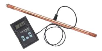
Copper Coating Thickness: All 100% rods (full production) are subjected to the coating thickness test. Every rod at several points is checked by an electronic thickness tester to measure the copper thickness on the steel core. The reading in case of UL listed rods is not less than 254µM and for other rods as specified by the end user.
